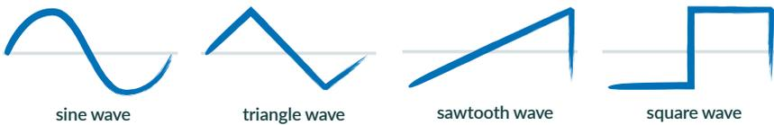
For instance, a sine wave oscillator produces a pure but dull tone, while a square wave sounds much harsher and has a very rich harmonic content.
