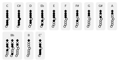
In addition, the left pinky key on the Sylphyo acts as a universal # (sharp) key, adding a semitone to any fingering, and the right pinky key acts as a universal b (flat) key, removing a semitone from any fingering.
